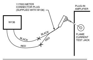
IF 117053 METER CONNECTOR PLUG IS NOT AVALIABLE (R7289A RECTIFICATION AMPLIFER ONLY)
